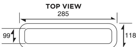
Dimension in mm Tolerance: ±0.03
